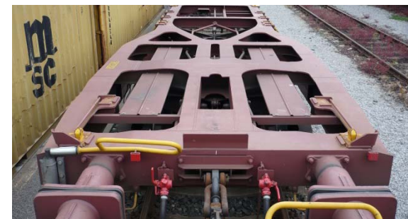
Light-weighted waggons with modern braking system
